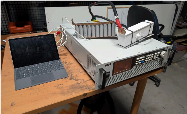
Discharge on a programmable electronic load.
